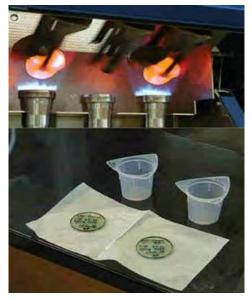
Petrochemical work often results in the total destruction of the existing minerals. Fusion into a glass is often required and commonly the most trusted method.
