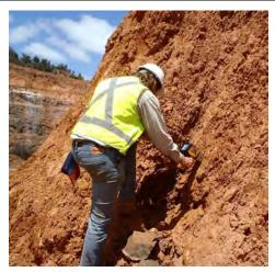
Using field-portable analytical devices, such as a hand-held XRF, have the advantage of speed, cost savings and convenience; however, reduced accuracy and precision as well as limited elements that can be detected make them a semi-quantitative device and generally unsuitable for most lithogeochemistry.
